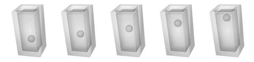
Figure 4: Single bubble rising in a continuous phase, for  $t = 0.015 \ s$ ,  $t = 0.030 \ s$ ,  $t = 0.045 \ s$ ,  $t = 0.06 \ s$  and  $t = 0.075 \ s$ . Here, Re = 30 and Eo = 2.
