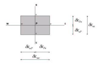
Figure 1: Two-dimensional control volume.
