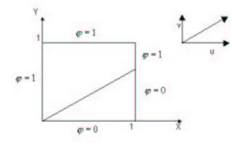
Figure 3: Illustration of the skew-convection diffusion problem.
