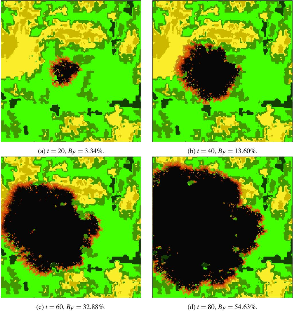
Figure 11: Experiments considering wind  $\vec{w} = 10$  direction east-west.
