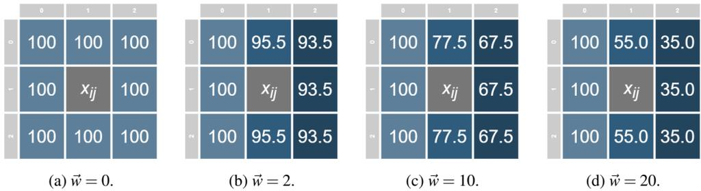
Figure 3: Fire spread was considered using a wind preference matrix inspired by the works of Schadschneider [18] and Lima & Lima [13].
