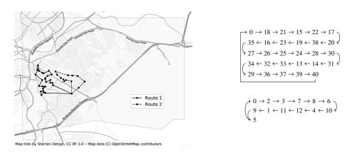
Figure 17: Routes minimizing FCR for Friday. 46 collection points are covered, totaling a distance of 9568.617 m, 54.544 kg of emitted  $CO_2$  and a FCR cost of R\$ 3.510. Numbers in nodes refer to Table A.5.
