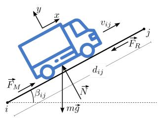
Figure 1: Forces acting on a truck moving upwards. Source: Adapted from [21].
