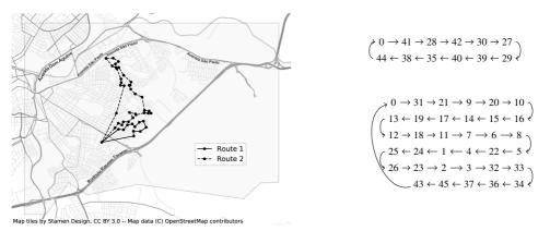
Figure 10: Routes minimizing  $CO_2$  emissions for Wednesday. 46 collection points are covered, totaling a distance of 9606.025 m, 54.400 kg of emitted  $CO_2$  and a FCR cost of R\$ 3.516. Numbers in nodes refer to Table A.3.
