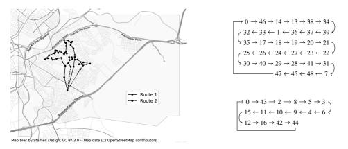
Figure 7: Routes minimizing  $CO_2$  emissions for Tuesday. 49 collection points are covered, totaling a distance of 10576.397 m, 61.394 kg of emitted  $CO_2$  and a FCR cost of R\$ 3.903. Numbers in nodes refer to Table A.2.
