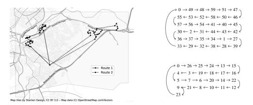
Figure 6: Routes minimizing distance for Monday. 60 collection points are covered, totaling a distance of 17932.364 m, 108.493 kg of emitted  $CO_2$  and a FCR cost of R\$ 6.721. Numbers in nodes refer to Table A.1.
