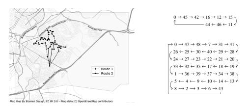
Figure 9: Routes minimizing distance for Tuesday. 49 collection points are covered, totaling a distance of 10560.528 m, 69.564 kg of emitted  $CO_2$  and a FCR cost of R\$ 4.069. Numbers in nodes refer to Table A.2.
