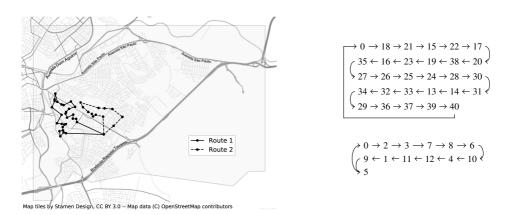
Figure 18: Routes minimizing distance for Friday. 46 collection points are covered, totaling a distance of 9490.884 m, 66.614 kg of emitted  $CO_2$  and a FCR cost of R\$ 3.755. Numbers in nodes refer to Table A.5.
