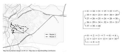
Figure 16: Routes minimizing  $CO_2$  emissions for Friday. 46 collection points are covered, totaling a distance of 9606.025 m, 54.400 kg of emitted  $CO_2$  and a FCR cost of R\$ 3.516. Numbers in nodes refer to Table A.5.
