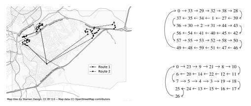
Figure 4: Routes minimizing  $CO_2$  emissions for Monday. 60 collection points are covered, totaling a distance of 17932.364 m, 104.993 kg of emitted  $CO_2$  and a FCR cost of R\$ 6.694. Numbers in routes refer to Table A.1.
