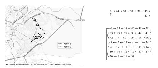
Figure 12: Routes minimizing distance for Wednesday. 46 collection points are covered, totaling a distance of 9490.884 m, 66.614 kg of emitted  $CO_2$  and a FCR cost of R\$ 3.755. Numbers in nodes refer to Table A.3.
